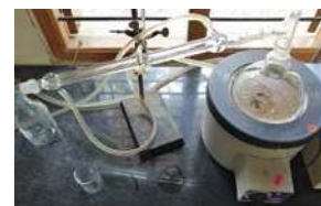
Fig 3: distillation process in laboratory
