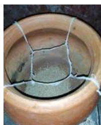
Fig 6: Lower mud pot with raw Ajamoda and cotton threads for hanging the collecting vessel.
