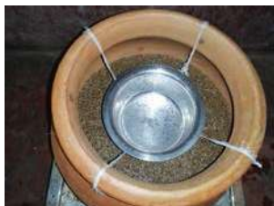
Fig 7: Lower mud pot with Ajamoda and collecting vessel.
